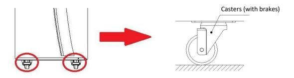
When the machine is moved on an uneven surface or with steps, four or more people are required to lift the machine to ensure safety.
