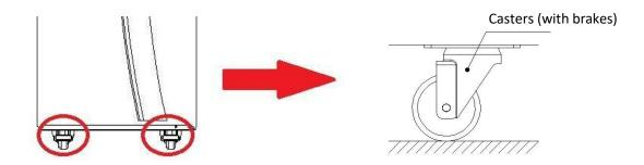
When the machine is moved on an uneven surface or with steps, four or more people are required to lift the machine to ensure safety.
